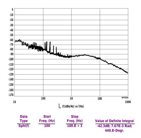
Integrated Noise WJ-8609A Tuned to 500.55 MHz at SM Out 70 MHz [hp] 3048A Carrier: 70.E  $\pm$ 6 Hz
